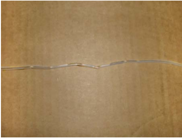
Figure 26: Typical Bad Membrane. Note the kinks and flat spots.
