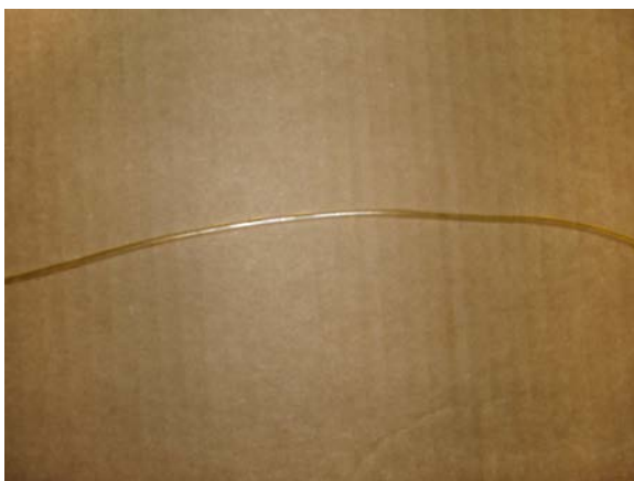
Figure 25: Typical Healthy Membrane
