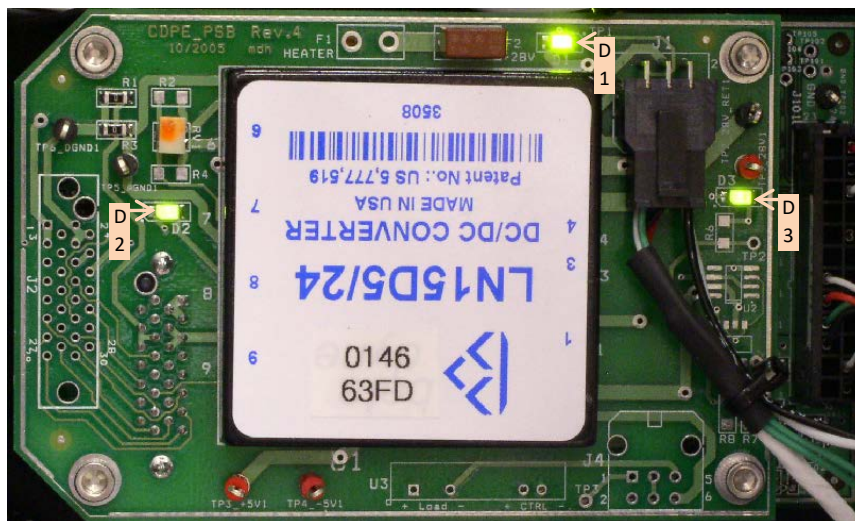
Figure 11: CDPE Board. D1, D2, and D3 are lit all the time when there is power supplied to the instrument
