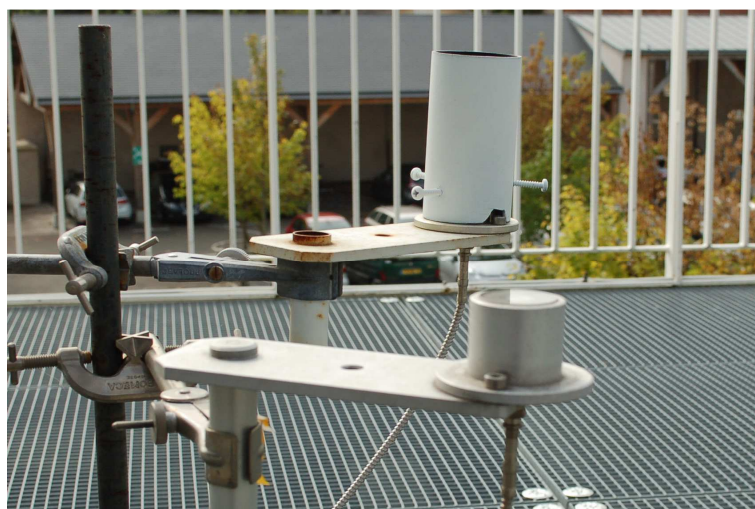
Fig. 2 Optical head equipped with a tube (white) for stray light protection and without a tube (grey).
