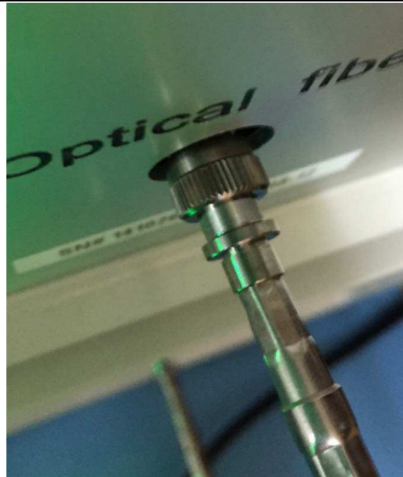
Fig A6-6: Optical fibre well connected, the screw thread is invisible
