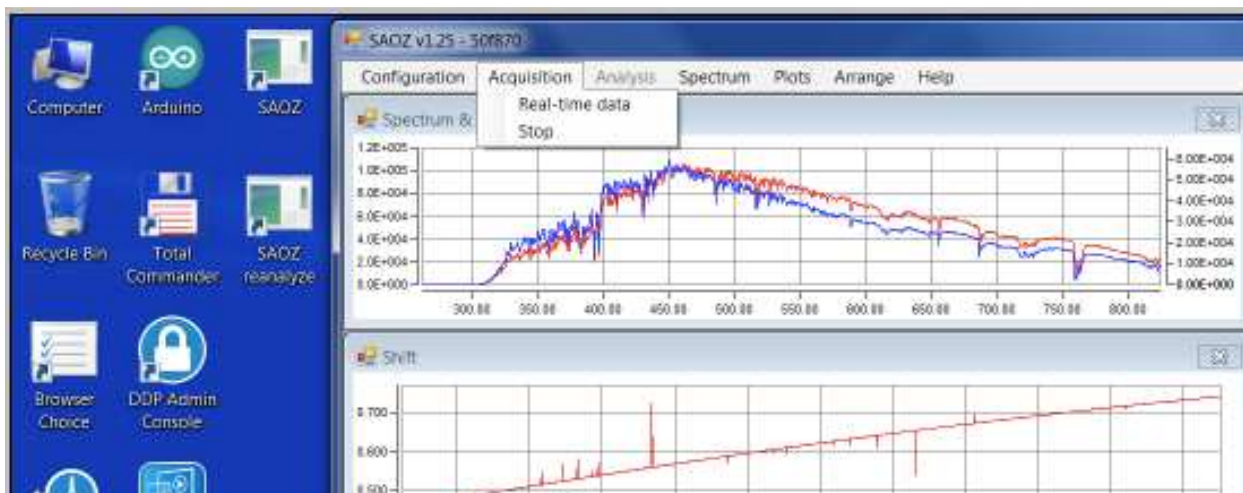
Fig. 4 SAOZ software screen to STOP (quit) the Real-time mode.
