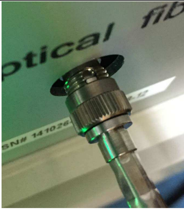
Fig A6-5: Position the fibre lug in the notch of the connector on the instrument and optical head side.
