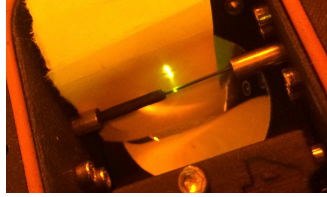
Figure 12. Example of a well-aligned laser beam, with alignment filament passing from the exhaust tube (right) to the inlet nozzle (left).
